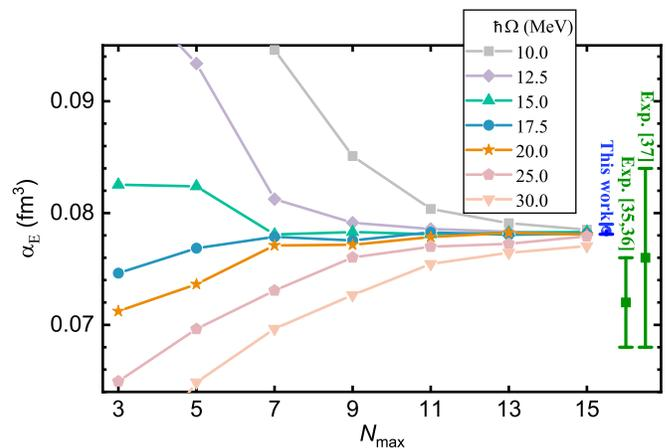
FIG. 3. (Color online) Electric dipole polarizability of  ${}^4\text{He}$  as a function of  $N_{\text{max}}$  for various  $\hbar\Omega$  values. The solid dot with an error bar represents the converged result with an estimated uncertainty. Two experimental data along with their quoted uncertainties (solid squares) from Refs. [35–37] are shown for comparison.
