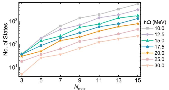
FIG. 1. (Color online) Number of  $1^-$  states in  ${}^4\text{He}$  up to the excitation energy of 100 MeV as a function of  $N_{\text{max}}$  calculated by the NCSM using the Daejeon16  $NN$  interaction with the Coulomb interaction between protons.
