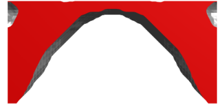
Figure 5: Design domain for an externally pressurized structure. The pressure load is applied on the top surface. The bottom, front and back faces get zero pressure loading. The left and right edges of the bottom face are fixed. The left and right faces slid in the vertical direction.
