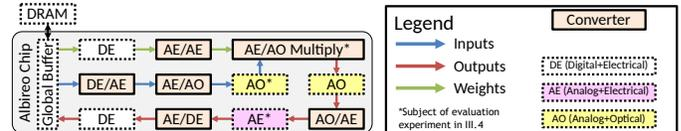
Fig. 1. Albireo architecture. As data traverse the DE, AO, and AE domains, they leverage different movement and reuse opportunities but pay energy for data converters, notated  $X/Y$  for conversion from domain  $X$  to domain  $Y$ .
